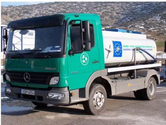
**Collection truck of Patras Transfer station with a storing capacity of 5.5MT**
